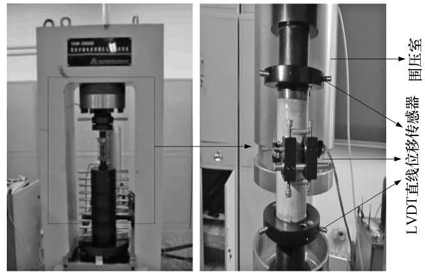
图1 微机伺服岩石三轴试验机 TAW-2000 Fig.1 Micro-computer servo rock triaxial testing machine TAW-2000
